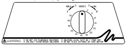
**Note:** In order to maxima the cleaning efficiency; it is always a good idea to "degas" the cleaning solution previous to real cleaning. This could be done by set the timer to 5-10 min. and let the cleaner run to allow solution to "degas".
