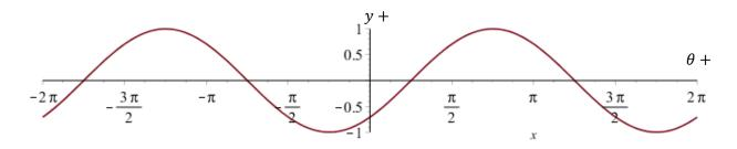
Finally, multiplying our angle by a constant will change the **wavelength** (distance from "peak-to-peak" or "trough-to-trough") of our wave. If we graph  $y = \sin(4\theta)$ , our resulting wave will have a wavelength that is  $\frac{1}{4}$  the length of our  $y = \sin\theta$  graph.
