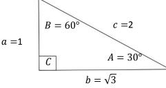
This standard 30-60-90 triangle serves to illustrate the concept of relating the ratios of a right triangle's sides to its angles. If we have a right triangle whose angle A is 30°, then we know the ratio of sides b to a must be  $\frac{\sqrt{3}}{2}$ , the ratio of sides a to c must to  $\frac{1}{2}$ , and b to c must be  $\frac{\sqrt{3}}{2}$ . Similarly, if we have a right triangle whose sides a, b, and c form these ratios, we know angle A **must be** 30°.
