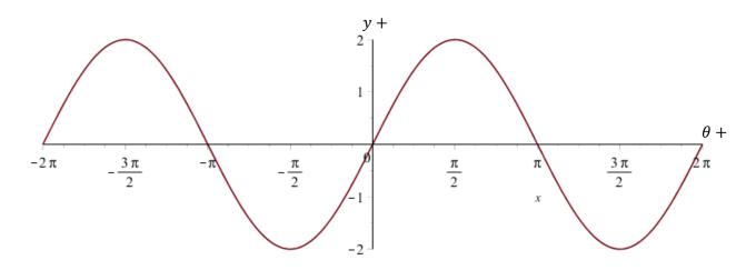
Adding a constant will shift our wave in the vertical direction. For instance, graphing  $y = 1 + \sin \theta$  will result in a wave shifted 1 unit in the positive vertical direction.
