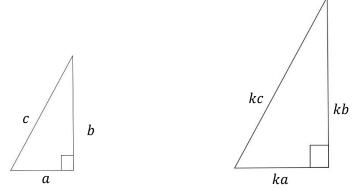
If we take the ratio of sides ka and kb on our larger triangle, we see that the constant coefficients cancel, and the ratio is equal to the ratio of sides a and b on our smaller triangle.
